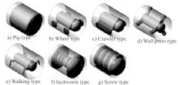
Fig 1. Classification of inpipe robots
