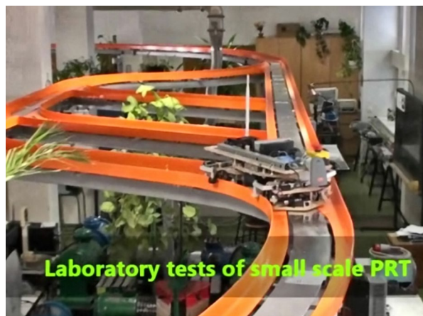
Fig. 1. Experimental track for studies of vehicle dynamics and motion control system operation
