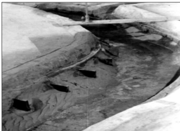
Fig 4. River bed regulation with river-training spurs (fragment of the Neris hydraulic model)
