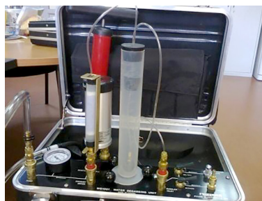
Figure 2. Experimental set-up diagram with the degassing system and Lucas cell coupling, and the laboratory experimental set-up
