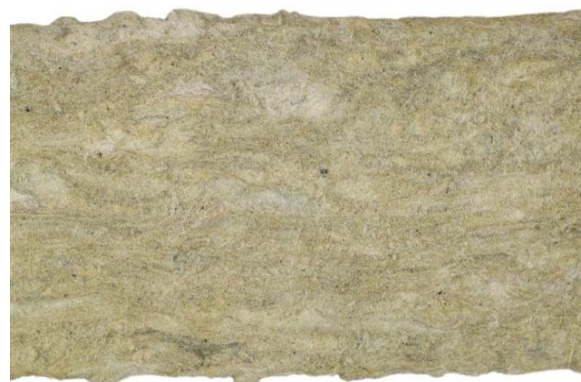
Fig 3. Distribution of fibres in the chaotic orientation of the stone wool slab structure (per product thickness)
