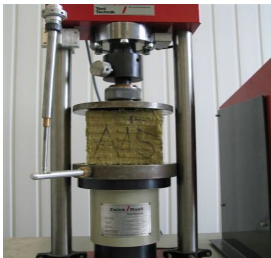
Fig 1. A specimen under load in the test machine “ToniNorm”
