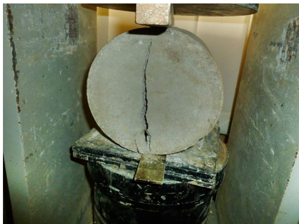
Fig. 2. Failure of cylindrical sample (Photograph by Author)
