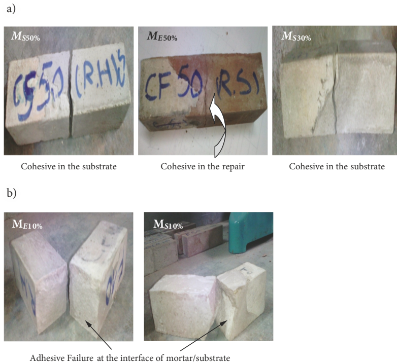
Figure 7. Failure mode on the mortar
