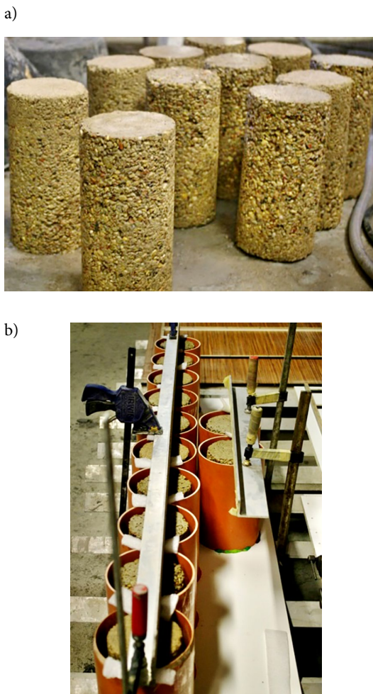
Figure 1. Preparation of specimens: (a) – surface after treatment with high pressure water jet; (b) – specimens in the moulds
